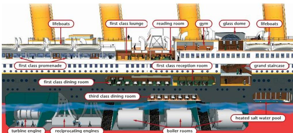
For safety reasons, the ship's steel hulls were divided into 16 separate compartments. She would stay afloat even if a massive hole was gouged in the side and two of the compartments were flooded. According to The Shipbuilder magazine, the Titanic was practically unsinkable.
